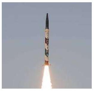
Agni-I was first tested at the Interim Test Range in Chandipur at 7:17 AM on 22 May 1989 and was capable of carrying a conventional payload of 1,000 kg (2,200 lb) or a nuclear warhead. Agni missiles consist of one (short range) or two stages (intermediate-range).
